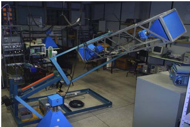
FIGURE 2. General layout of the Tupi telescope, constituted by four scintillator detectors, of which two are installed in coincidence and forming a tracking telescope.
